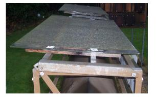
discolouration and a "tiger stripes" assess this phenomenon, ECCA has developed techniques. an outdoor test method to evaluate dirt pickup along with the cleanability of painted surfaces.
